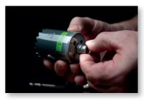
Screw the supplied adapter onto the holesaw.
